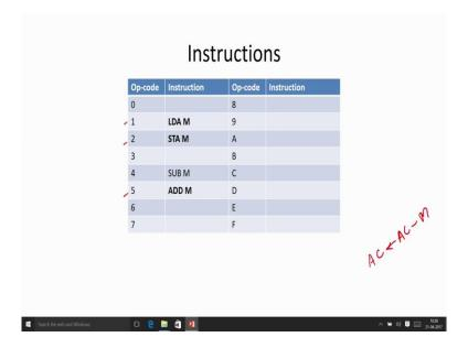
these 3 Instruction. Now, we are saying that we are designing one more Instruction call SUB M. So, it means subtraction. So, what is this Instruction this is basically nothing but Accumulator is equal to Accumulator minus contents of the Memory. Ok we are going to give the Instruction format is same whatever we are going to design for all the Instruction it is going to follow this particular pattern.
