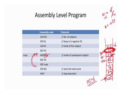
Or assembly level, I can say like that. So, this is basically related to this particular example. Here we are saying what first I am writing load Accumulator M1.
